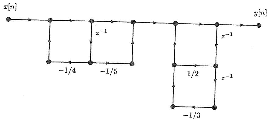
(iv) Parallel form using first and second order direct form II sections.
