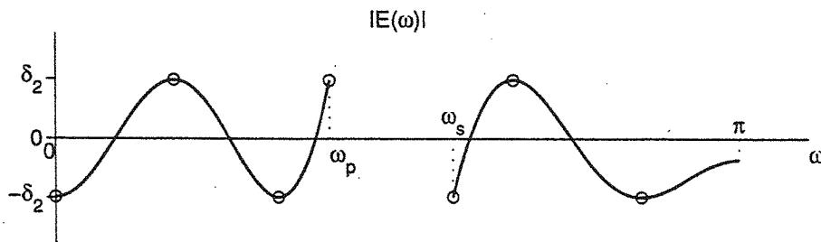
(d) An optimal (in the Parks-McClellan sense) Type I lowpass filter can have either  $L + 2$  or  $L + 3$  alternations. The second case is true only when an alternation occurs at all band edges. Since this filter does not have an alternation at  $\omega = \pi$  it should only have  $L + 2$  alternations. From the figure, we see that there are 7 alternations so  $L = 5$ . Thus, the filter length is  $2L + 1 = 11$  samples long.
