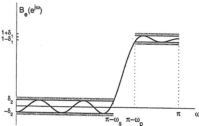
(d) The assertion is correct. The original amplitude function was optimal in the Parks-McClellan sense. The method used to create the new filter did not change the filter length, transition width, or relative ripple sizes. All it did was slide the frequency response along the frequency axis creating a new error function  $E'(\omega) = E(\omega - \pi)$ . Since translation does not change the Chebyshev error ( $\max |E(\omega)|$ ) the new filter is still optimal.
