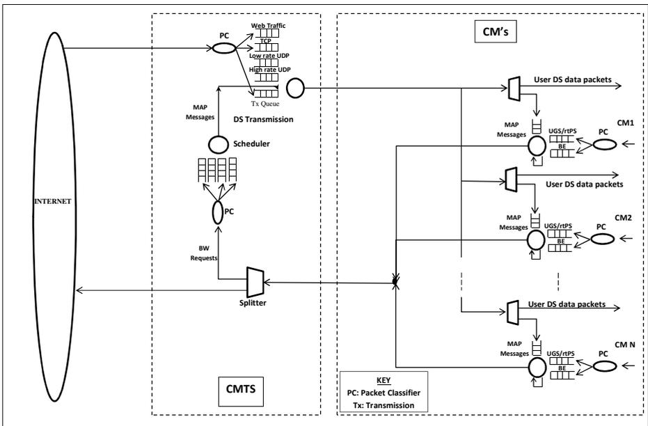
Fig. 5. Simulation delay model
