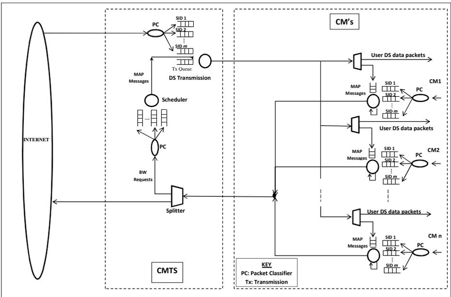
Fig. 3. QNM of a general DOCSIS 1.1/2.0 HFC network
