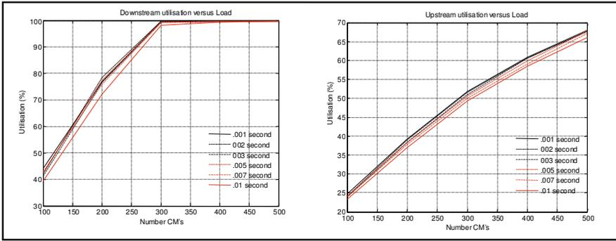
**Fig. 11a.** Downstream channel utilisation (Experiment set II)
