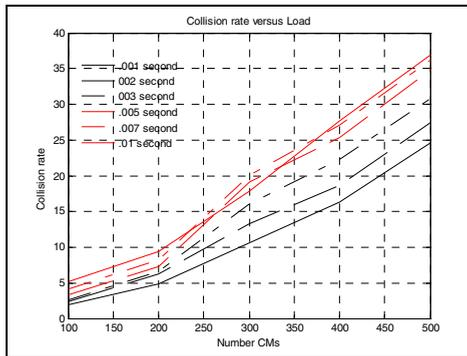
**Fig. 10.** Upstream collision rates. (Experiment set II).
