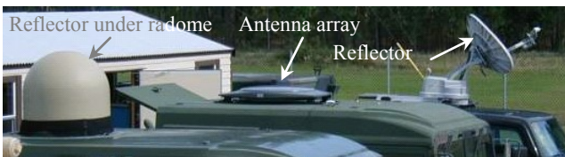
Fig. 2. Visible importance of the low-profile antennas for ground vehicles
