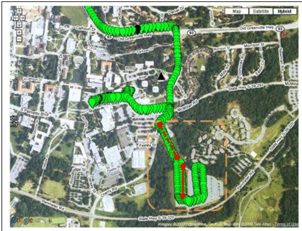
Figure 2. Coverage Data from 2/15/2009 (Basestation Identified by the Black Triangle)
