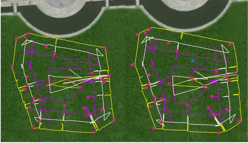
Fig. 9. Trajectories of three UAVs in field test (left) and simulation environment (right) when completing a task with 30 points.
