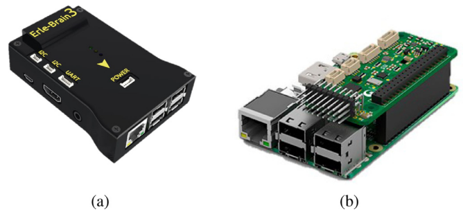
Fig. 7. Erle-Brain autopilot: (a) Erle-Brain 3 (b) PXFmini on top of a Raspberry Pi.
