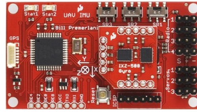
Fig. 13. UAV Development board v3 from Sparkfun used by the MatrixPilot.
