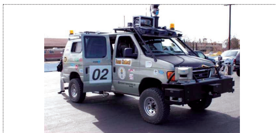
Figure 1. Alice, Team Caltech's entry in the 2007 DARPA Urban Challenge. The Ford Econoline van was equipped with 10 cameras; eight laser radars (LADARs); two ordinary radars; an inertial navigation system; two pan-tilt units; 25 CPUs; and actuators for the steering, throttle, brake, transmission, and ignition.
