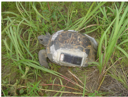
Fig. 1. A solar-powered tracking device used in TurtleNet.
