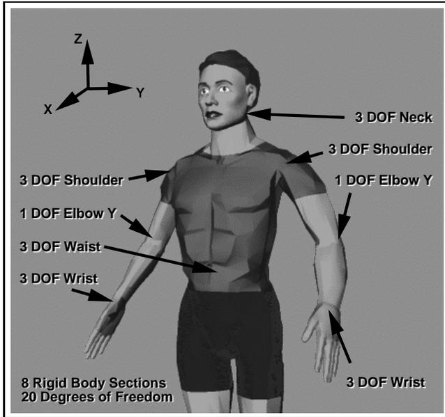
Figure 3: *The Adonis 20 DOF full-body dynamic simulation.*
